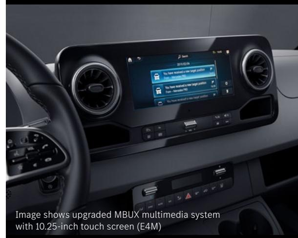
Image shows upgraded MBUX multimedia system with 10.25-inch touch screen (E4M)
