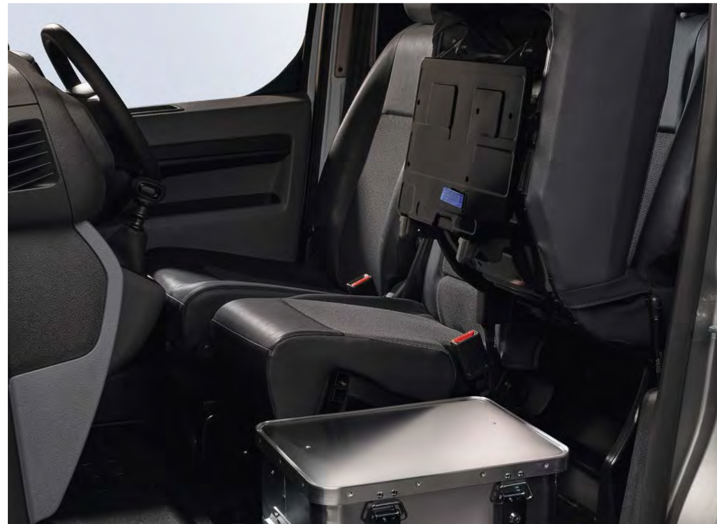
Load-through hatch within bulkhead.
