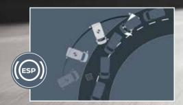
Electronic Stability Program helps detect and automatically correct skids by sensitively braking individual wheels. A load detection system compensates for the weight of your cargo.
