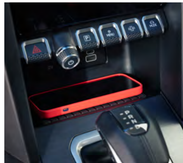
Function keys as well as an on/off button and volume control for the infotainment system (from the Style onwards with chrome-look surround), 12-volt socket, USB-A and USB-C interface, and a mobile phone storage compartment (from the Style onwards with inductive charging function, otherwise optional) in the storage compartment below the touch colour display.
