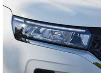
LED low beam, turn indicator and Daytime Running lights
