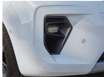
LED front fog lights with cornering technology [1]
