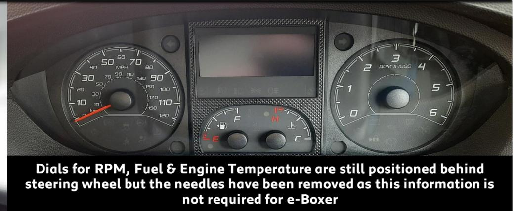
Dials for RPM, Fuel & Engine Temperature are still positioned behind steering wheel but the needles have been removed as this information is not required for e-Boxer
