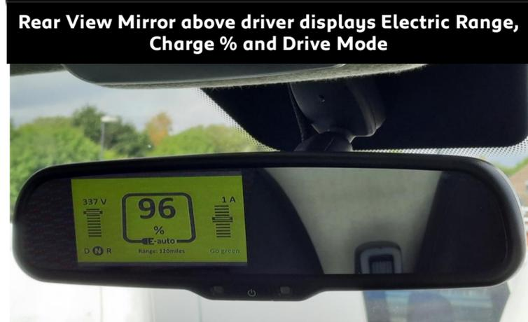
Rear View Mirror above driver displays Electric Range, Charge % and Drive Mode
