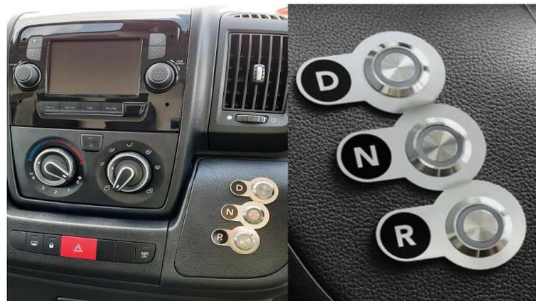
Gear Lever replaced with Drive Mode select buttons located to the left of the steering wheel
